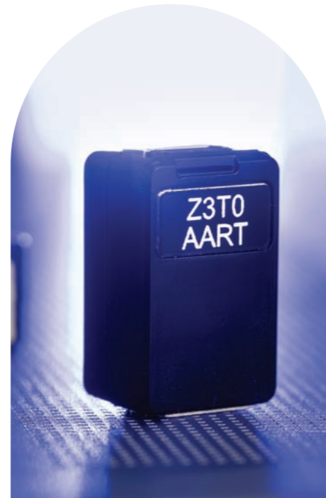
A quantum sensor. These lego-brick sized devices exploit the quantum properties of Rb atoms to measure magnetic fields.
