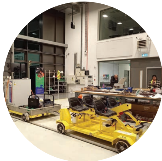
Preliminary testing of a mobile stabilisation platform setup at the National College for Advanced Transport & Infrastructure in Birmingham, UK. The platform (rear), control unit (centre) and drive cart (front) were investigated for vibrational characteristics along a section of railway in preparation for the deployment of quantum sensors.
